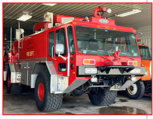
gallons of water, has a pump capable of 1,250 gallons per minute, has a bumper turret (300 gpm), and a roof turret (750 gpm), and is equipped with foam.
