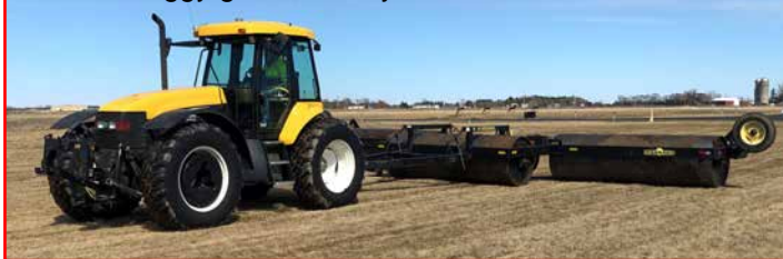
The 145 horse power New Holland TV145 smoothing out the soggy grass runway in March of 2019
